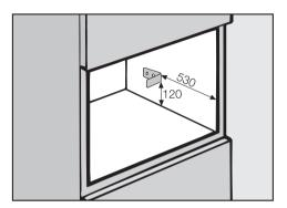
Secure bracket (A) using screw (B) in the position shown inside the housing unit.
